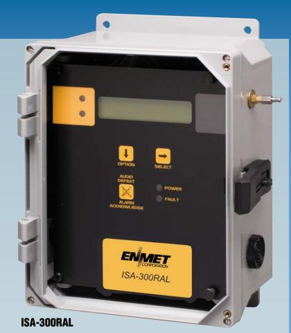
The ISA-300RAL respiratory air line monitor automatically and continuously monitors compressed air lines for CO and activates audio and visual alarms if the concentration of the contaminant rises above preset limits. The instrument is designed to alarm at a concentration of 10 ppm CO in Grade D breathing air as specified by Federal OSHA guidelines. (5 ppm in Canada, per CSA Z88)
